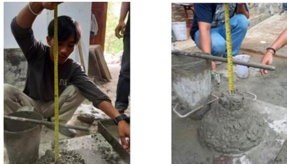
Gambar 2. Proses uji slump
