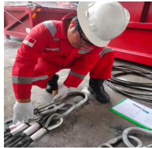
Gambar 6 : Visual Inspection Wire Rope ID Number: 22080095-001
