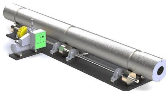
**Gambar 5. Varian 2 mesin *centrifugal casting***
