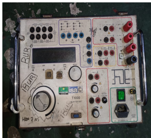
Gambar 7 Alat Uji Test Proteksi Relay
