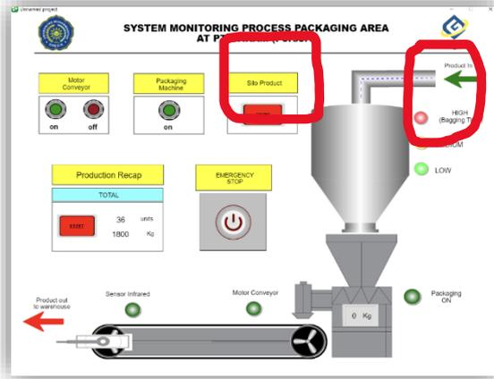
Gambar.13 Tampilan HMI Saat Membaca Level isi Silo
