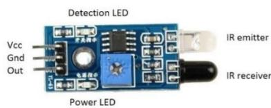
Gambar.5 Sensor Infrared
