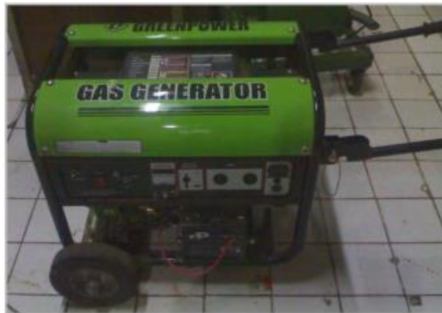
Figure 2.1. LPG engine-generator set used in the experimental study (placeholder).
