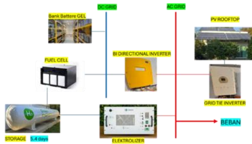
Figure 9. PV BESS Hydrogen Combination
