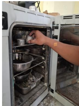
Picture 1 Water Content Testing
