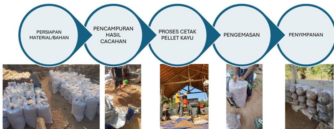
Figure 1. Scheme and Documentation of Wood Pellet Production
